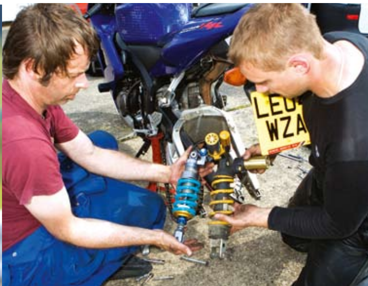
Above: Al and Ben make a shock change look easy. Sort of Right: Lightweight, CNC machined, aircraft alloy shock with third piston shim stack for very low rebound control
