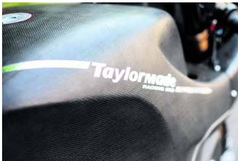
Tank surround (above) is part of monocoque frame. A-frames let forks deal with bumps, not braking forces
