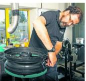
**Laying out** Bike carbon wheels are laid out by hand in a mould in two halves, with ten layers of carbon, Kevlar and resin.
