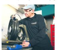
**Trimming** Carbon wheels are 'deflashed', trimmed and polished by Bryan. The finish is pure carbon.
