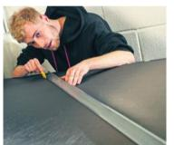
Raw carbon Tyler Lynch cuts some of the UK-supplied raw carbon for a wheel. A kit of parts then goes to the laying out area.
