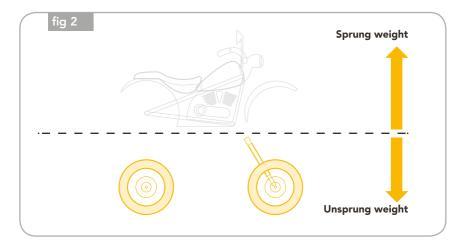
When a bike passes over a bump in the road, the rider will feel the unsprung weight being forced upwards. At high speeds this causes unpleasant vibrations - the greater the bike's unsprung weight, the stronger these vibrations become.
