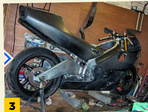
MAR 2015 - THE REAL DEAL The bodywork doesn't just look like Mick D's - it's from the very same HRC moulds. Made in carbon by CTech Composites.
