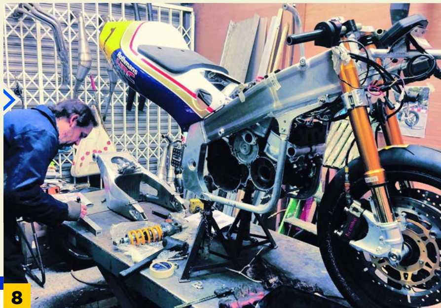
MAY 2015 - BACK (END) IN THE GAME The swingarm may be Yam R6, but all the linkages and shock mounts are bespoke to match the dimensions set out by 2moto's Felix Hirzel, who designed the chassis. Note the mount, behind the swingarm pivot, for the adjustable 2moto footrests.
