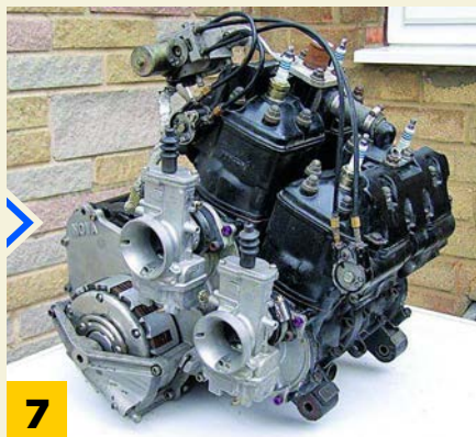
APR 2015 - RACE READY Stage 3 RG500 motor with Nova 'box and dry clutch. Makes 100bhp in road trim; good for 120bhp with saucy disc valves...
