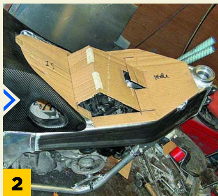
MAR 2015 - CUT IT OUT The business end is neatly tucked away under an aluminium cover, which Barry made first as a cardboard template.
