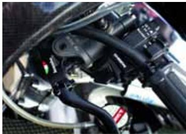
Radial master cylinder is Brembo 16 RCS
